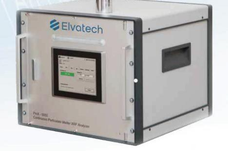
PmX-5050 is a Continuous Particulate Matter XRF Analyzer intended for online elemental analysis of heavy metals in the ambient air.
