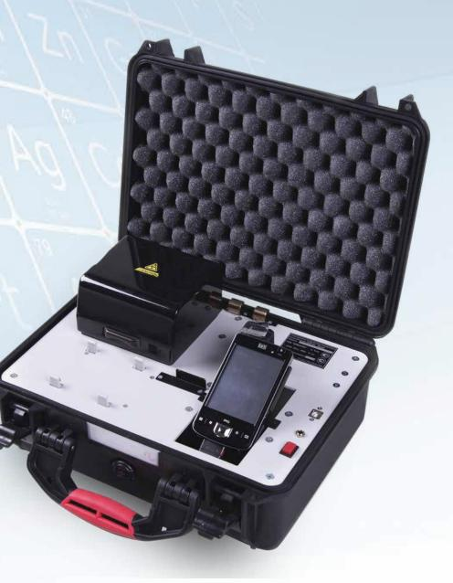
ElvaX Mobile is a portable EDXRF analyzer for testing a wide variety of materials.
