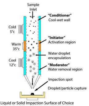
The Spot Sampler collector uses a patented, three-stage "moderated" condensational system to enlarge aerosol particles and then gently deposit them by inertial impaction.
