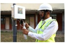
On-site calibration of Oizom devices can be performed using standard calibration gas cylinders of known concentration or by co-locating with a reference standard.
