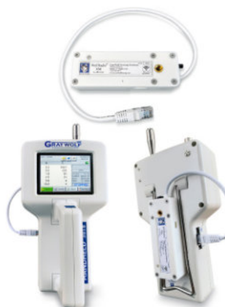
Optional WOLFRADIO-XM-3016 wireless module adds Bluetooth and Wi-Fi (for WolfOS, Android, iOS, and cloud connectivity)
