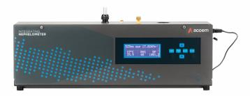
The Aurora 2000 PM<sub>2.5</sub> Correlating Nephelometer is part of the new generation nephelometers, using a single wavelength and an LEDlight source to measure aerosol light scattering and derive particulate concentrations.
