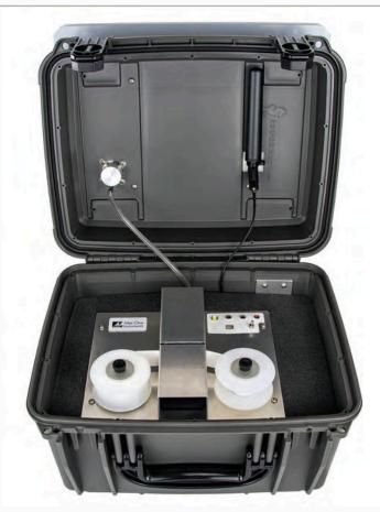
The C-12 is an industrial-grade device, providing the user with an array of diagnostic information in real-time that will allow them to monitor its performance continuously. Although it is inexpensive compared to other commercially available carbon monitors, one can expect its operating life to be more than ten years.
