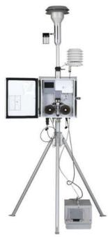
The E-BAM Plus is a portable, real-time beta gauge built to satisfy users, regulators and those from the health community by providing truly accurate, precise and automatic measurement of fine particulate matter. (Accuracy exceeds US EPA PM<sub>10</sub> FEM requirements, range 0 to 10 mg/m³.)
