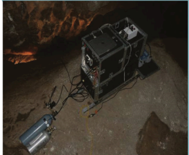
Figure 8. Spectronus™ was involved in a preliminary study of trace gas variations in limestone caves in 2008. 6
