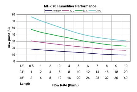
The above performance curves are for the MH-070. The MH-110 gives roughly a 3 degree higher outlet dew point than the MH-070. The MH-110 should be selected when a lower pressure drop is desired.
