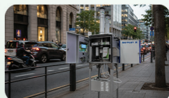
Medium-volume samplers (10-50 L/min)
